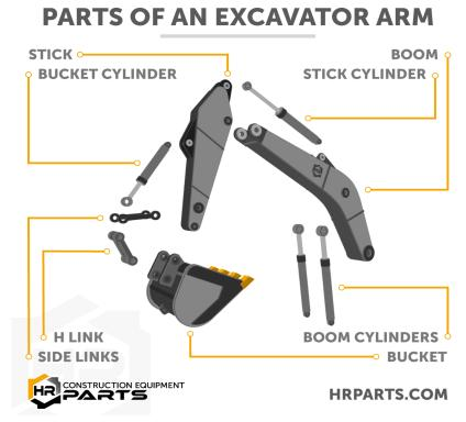
3. **Attachment/Bucket**: The attachment is the part of the machine furthest from the operator. that has the main purpose of holding material inside. Although there is a variety of attachments the most used attachment is the bucket.
